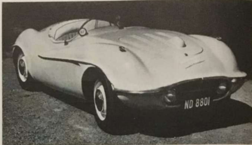
This view of the "Incorporated Special" shows well the wind-cheating lines of the car. The body was designed by Mr. Douglas Lindsay. With the special Alta "Birmidal" cylinder head, the engine develops 38 b.h.p.
